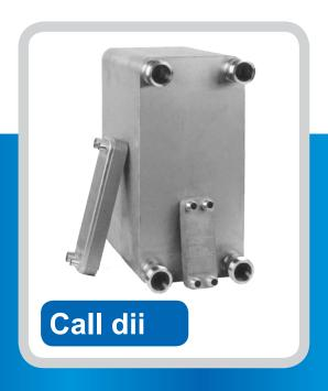
The compact size, low refrigerant charge, and superior heat transfer characteristics of Doucette's Brazed Plate Heat Exchangers make them ideal for evaporator, condenser and sub-cooler applications. Available for virtually any duty, the Brazed Plate Heat Exchangers are available with copper or nickel brazing materials. Standard units have 316 Stainless Steel plates with copper brazing and sweat connections. U.L. listed for 650 psig DWP.
